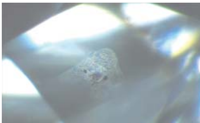
Dark inclusions of graphite in healed "fingerprint" were seen in this Bel-lataire diamond examined in 1999. Photomicrograph, magnified 15 times, by John Koivula, copyright GIA.
