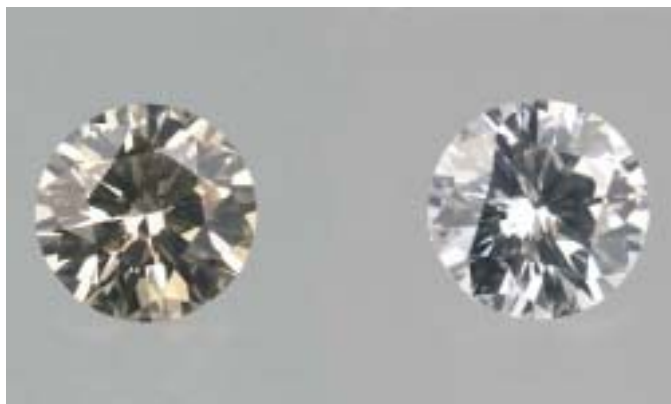
Taken before (left) and after (right) treatment of the same 1.01 carat type IIa diamond, these photos show the decolorization that can be produced by the HPHT process. Photographs by Elizabeth Schrader, copyright GIA.
