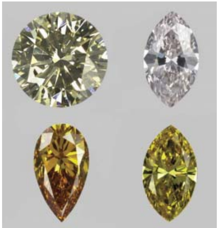
These four type Ia diamonds (0.30–1.89 carat) were HPHT treated in Russia. Photograph by Elizabeth Schrader, copyright GIA. Stones courtesy By Nature.
