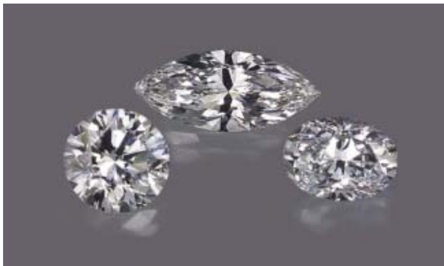
These three GE Bellataire type IIa diamonds (4.11–5.34 carat) are products of the HPHT process. Photograph by Elizabeth Schrader, copyright GIA.
