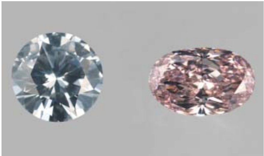
Blue (3.42 carat) and pink (1.72 carat) GE HPHT-processed type II diamonds. Photograph by Elizabeth Schrader, copyright GIA.
