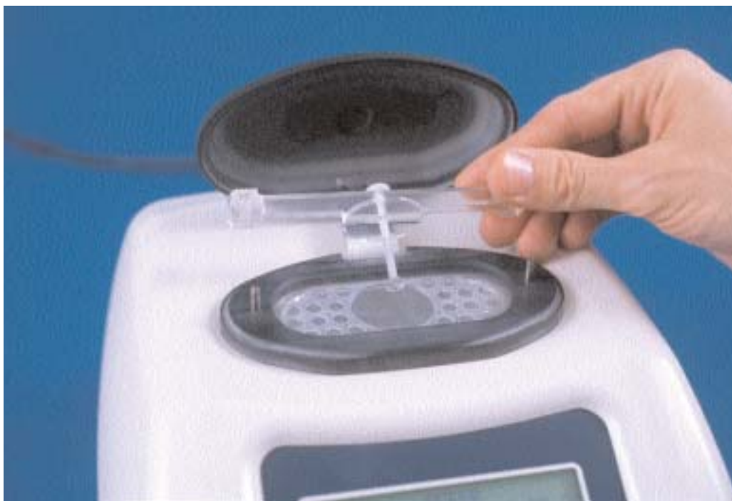
A diamond being inserted into liquid nitrogen containing a sample chamber of the prototype instrument designed for screening HPHT-treated type II diamonds.
